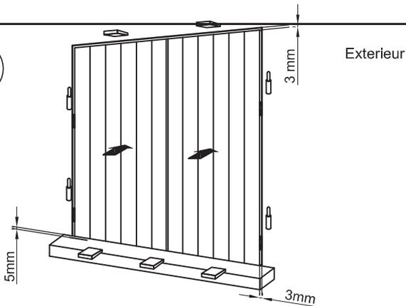
POSITIONNER LES VOLETS DANS LE TABLEAU AVEC DES CALES.
